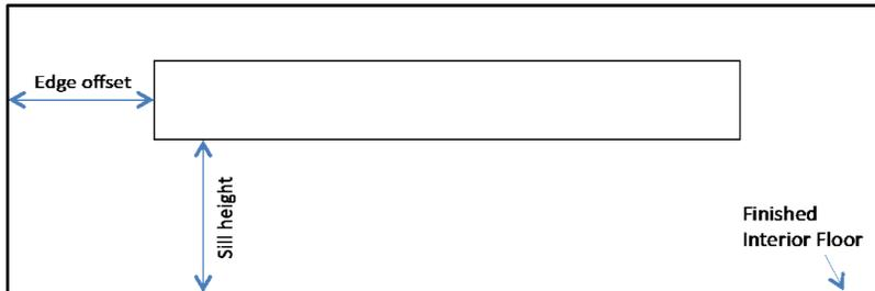
Discrete window layout—Enter the *number of windows* and the *width* and *height* of the windows per the following diagram, and the Tool will calculate the window-to-wall ratio:
