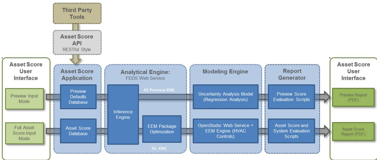
**Figure 4.2.** Asset Scoring Tool components.
