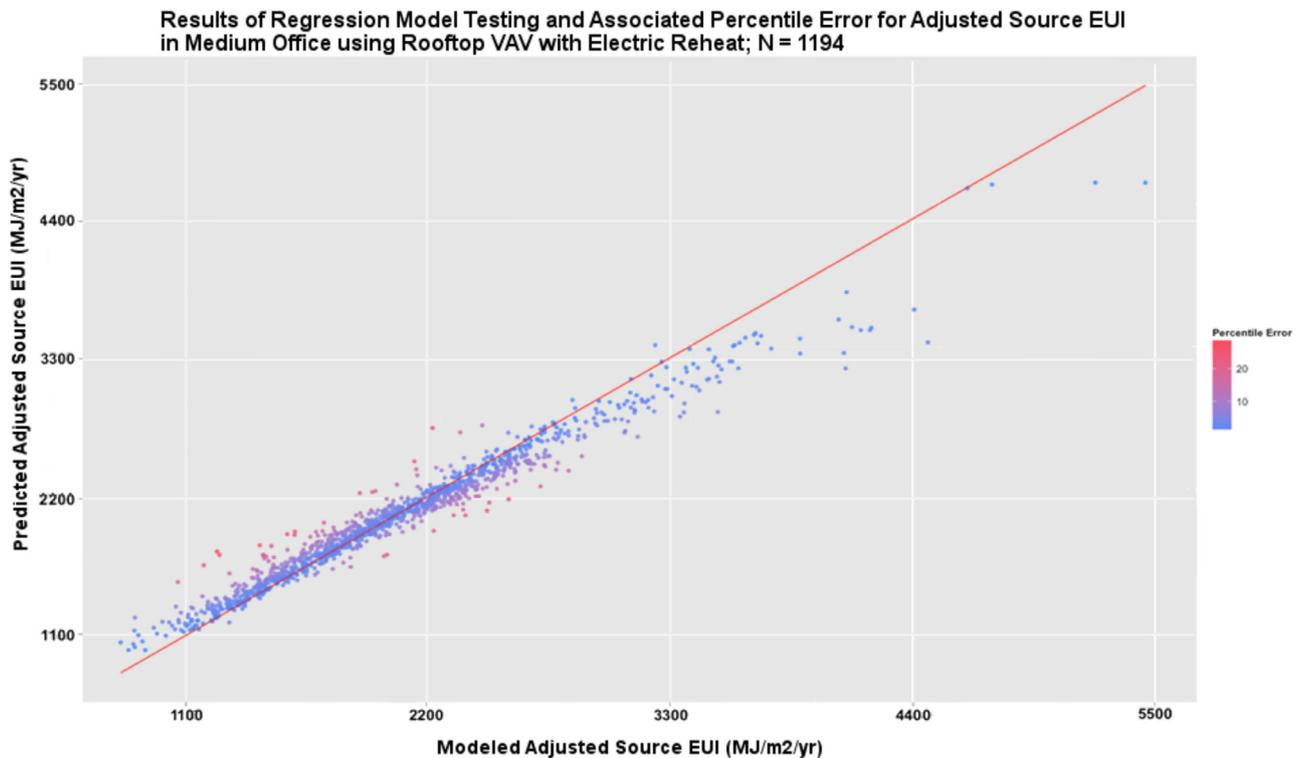
Fig. 6. Parity plot showing the fit of the reserved test data of 1194 data points against the predicted values of the regression model.
