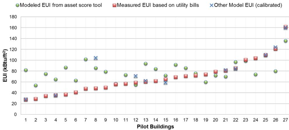
**Figure 2** Whole building site EUI (kBtu/sq.ft): Asset Score compared to utility bills and calibrated energy models
