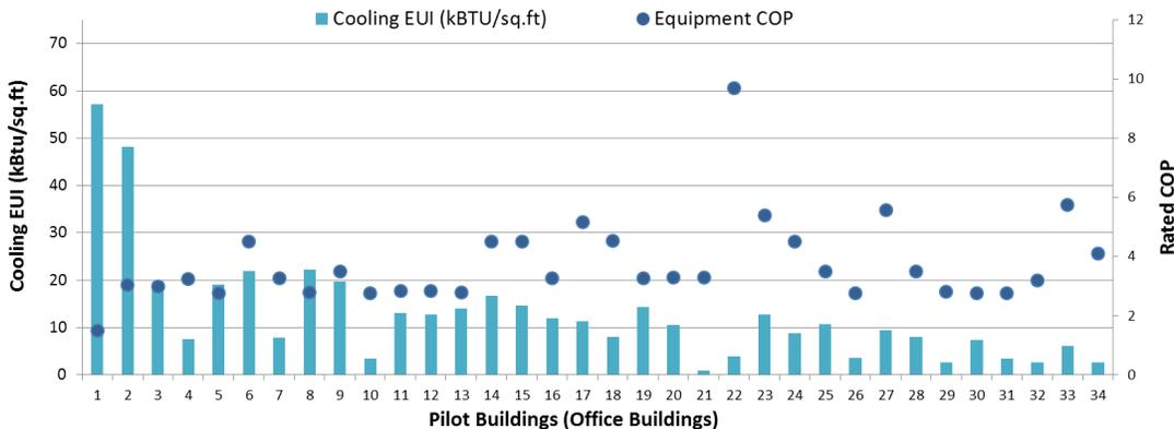
**Figure 4** (a) Cooling EUI (kBtu/sq.ft) vs Asset Score (b) Cooling EUI (kBtu/sq.ft) vs rated equipment COP (Note that the COP value for building No. 22 is incorrect because of user’s data entry error. An EER value was likely entered as COP.)
